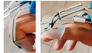
Fig. 1. Early prototype showing the device’s independence from changing CoRs of the index finger during flexion and extension
