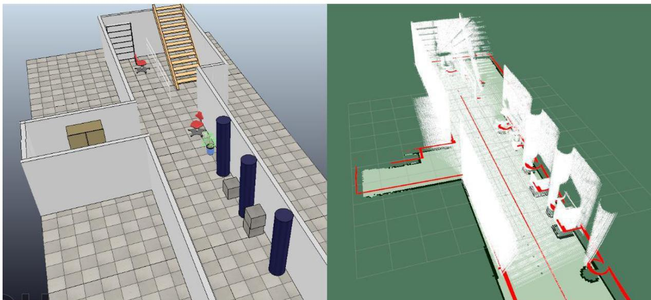
Fig. 4. (left) initial test scene created in VREP (right) Simulated 2D Lidar and depth sensor data combined in Rviz. Created by the mobile platform moving in a straight line in a single direction in simulation.
