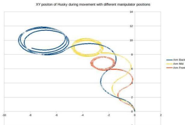
Fig. 3. Initial results showing XY position of the platform, with the same motor input, for 3 different manipulator mounting locations.
