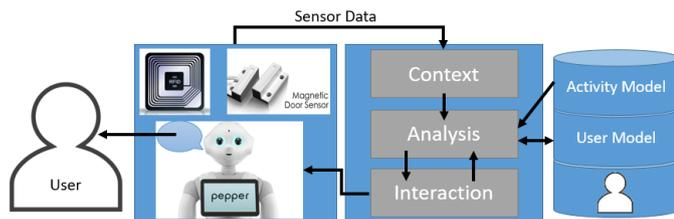
Fig. 1. Proposed architecture for automatic cognitive assessment
