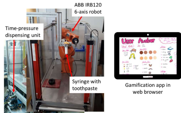
Fig. 2. Overview of the setup for the robotised dispensing experiment.
